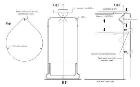
Assemble using the included flat-head screws
